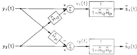
Fig. 3. The reconstruction system.
