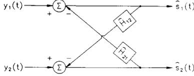
Fig. 4. An alternative implementation of the reconstruction system.
