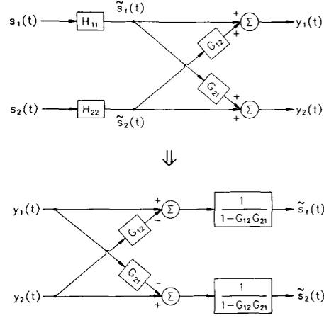
Fig. 5. The system for generating  $\tilde{s}_1(t)$  and  $\tilde{s}_2(t)$ .
